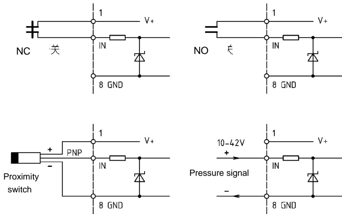
**Connection diagrams for switches and digital signal input**
