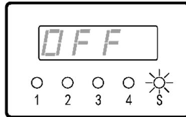
10. Press key
