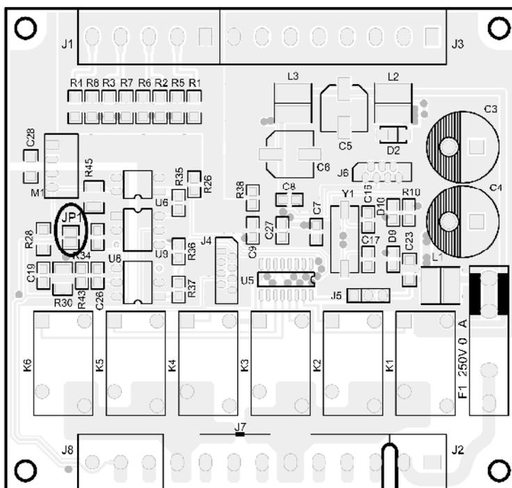
In order to make the network signal transmission stable, for longer network ( >300m ), especially network with less equipments, 120  $\Omega$  termination resistor has to be accessed to RS-485 interface of the first and the end control station.
