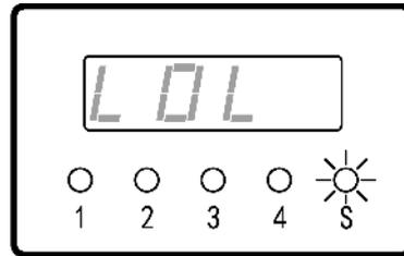
8. Press key
