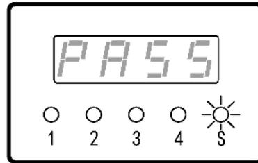
8. Press key
