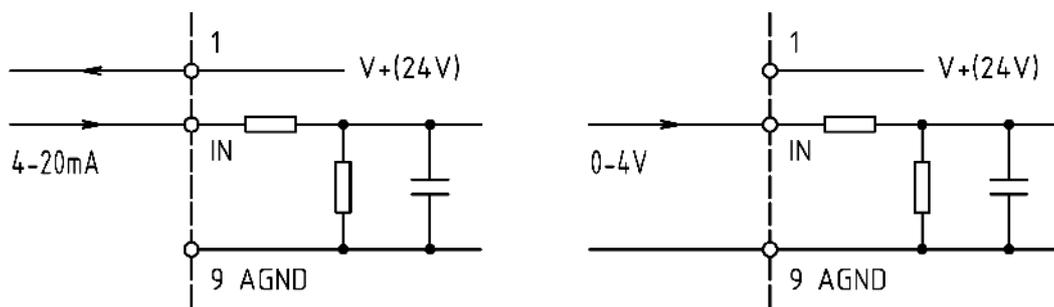
**Connection diagrams for analog signal input**
