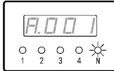
9. Press key
