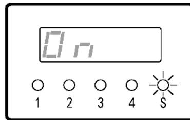
10. Press key
