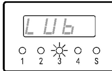
6. Press key
