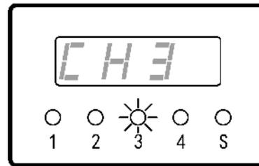
5. Press key
