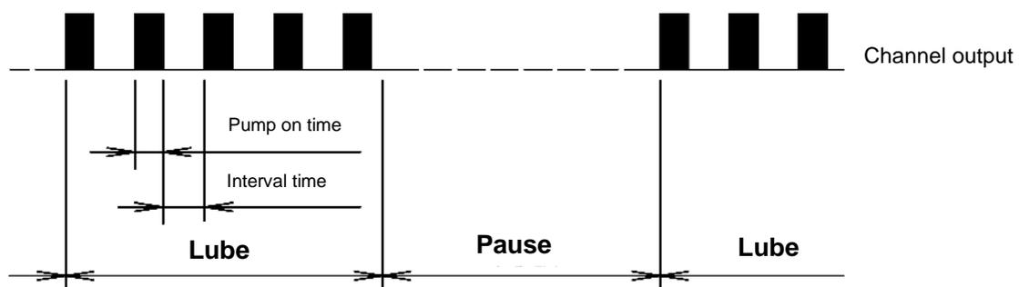
This lube mode is to send a series pulses to pump or oil feeder during lube
