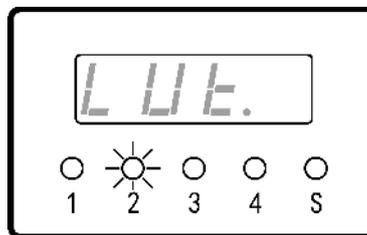
Inserted lubrication has very high priority. Unless system is halted ( or interlock open), user can start an inserted lubrication in any other states.
