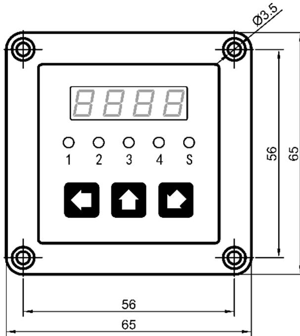
General panel component's installation method is different from UC-3N's special panel, but LED monitor, pilot lights and keyboard are all same. If users need to make opening on the box of their equipment to mount this panel, please refer to the panel CUT-OUT diagram as follow:
