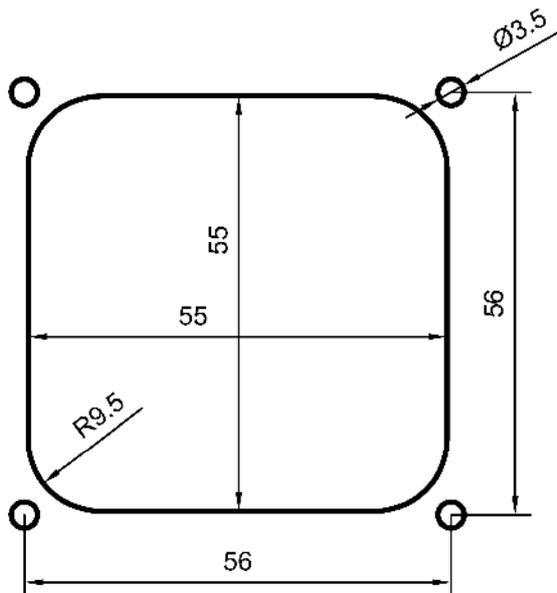
The 4 holes of  $\Phi 3.5$  on the four corners are all unthreaded holes. It is recommend to use machine screws for them. If users want to use self-tapping screws to install the panel, then make the bottom hole as  $\Phi 2.4$  and select ST2.9 self-tapping
