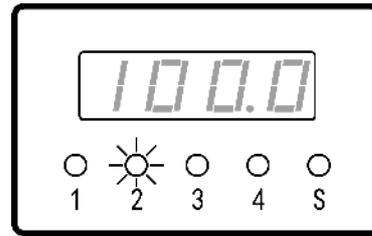
If it is LUt ( LUBE, timer ) state, then the measurement units of the displayed parameter is **second**.
