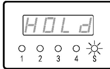
8. Press key
