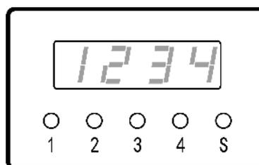
3. Press key
