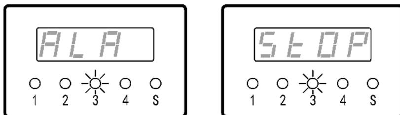
When any channel occur any faults, originally closed fault relay will open to send out remote fault indication.
