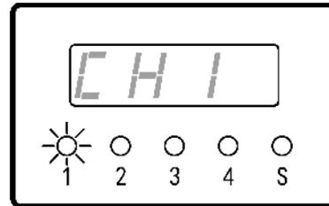
5. Repeatedly press key
