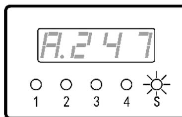
2. Press key
