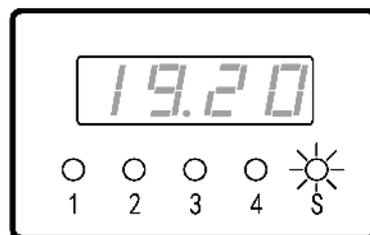
10. Press key
